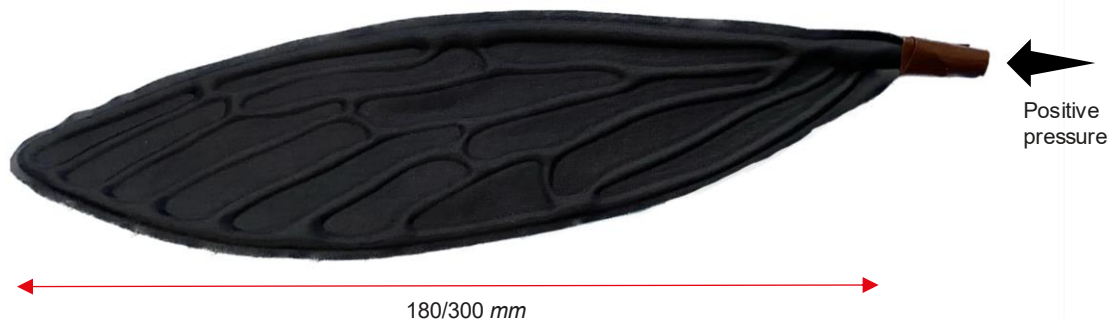
Figure 4: Heat Sealed TPU Coated Nylon Wing
